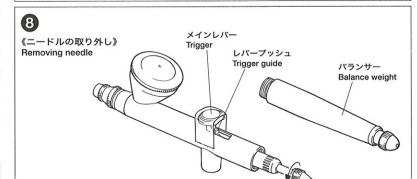
Cleaning inside the airbrush and cup: Clean paint from cup and wipe cup and cover using a rag. Fill cup with the appropriate thinner and attach cover. the fully loosen the needle stopper and block the nozzle tip with a rag. Allow air to flow from compressor/ can and pull the trigger. This will back flush air and thinner through nozzle and cup. Repeat this twothree times, using fresh thinner until all paint residue is eliminated.
